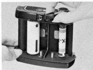
5. Move the film advance lever (R 3) gently, until the starting mark (arrow) of the leader paper aligns with the starting mark (R 12) of the holder. The film advance lever can be moved in several short, definite strokes.
