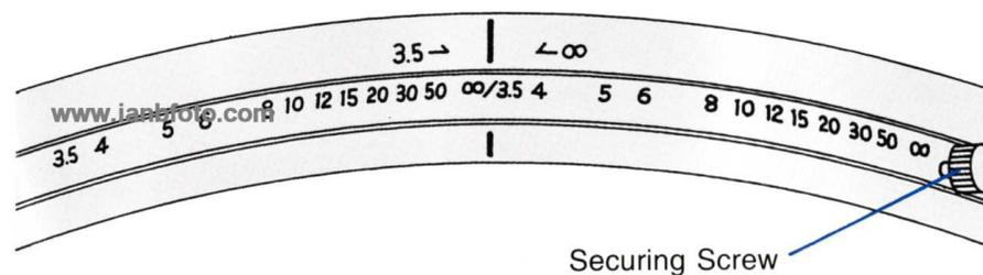
The left scale permits locking the most distant point of focus and restricts the lens from focusing past the point.
