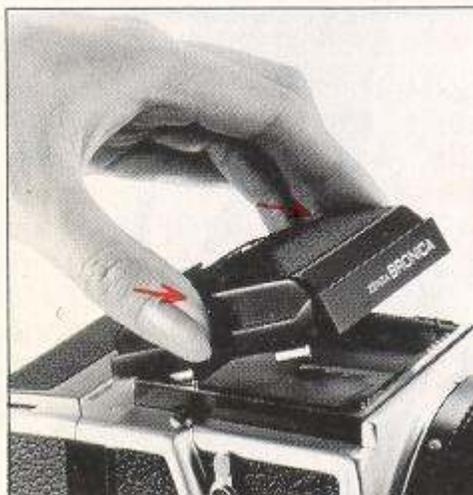
**B.** To attach the finder on the body, first, simply place protrusions on the bottom of the finder into corresponding openings in the finder frame and, then, slide the finder forward where it will lock.
