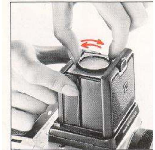
**C.** The standard magnifier supplied with the waist-level finder has a power of  $-1.50$  diopters, which can be exchanged for others with Powers of  $+1.50$ ,  $+0.50$ ,  $-0.50$ ,  $-2.50$ ,  $-3.50$  and  $-4.50$  diopters. These optional accessories should be purchased to suit the user's eyesight, if necessary.
