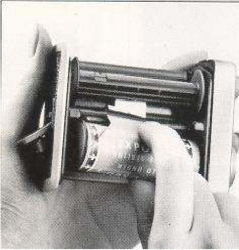
**A.** After the 15th exposure of the 120 roll film (30th exposure of the 220 roll film), the film winding crank will turn freely with further rotations. Therefore, continue rotating the film winding crank until the remaining film and all the leader paper is wound up on the take-up spool.
