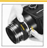
B. Then, slide the lens release button, in the arrow-indicated direction, and, at the same time, rotate the lens in the clockwise direction until it makes a full stop, at which point it will be possible to detach it.
