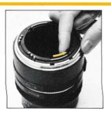
B. Since the cocking pins of the accessory will return slightly in the releasing direction, upon detachment from the body, move the cocking pins to their proper locations with your finger.
