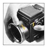
C. In order to detach the accessory from the body, press the lens release button (on the left side of the body) down and, at the same time, rotate the accessory in the clock-wise direction until it makes a full stop and can be detached.
