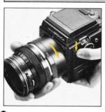
A. First, rotate the film winding crank and cock the shutter. Then, push the lens release button on the left side of the body down and, at the same time, rotate the accessory in the cockwise direction until it makes a full stop, at which point it will be possible to detach the accessory and lens.
