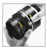
C. Next, rotate the lens release button of the accessory in the arrow-indicated direction and, at the same time, rotate the lens in the clockwise direction until it stops, at which point, it will be possible to separate the lens and accessory.
