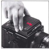
B. To attach the Waist-Level Finder G, simply align the front end of the finder with the finder frame (the shiny square frame on top), as illustrated. Then, gently lower the finder and, when well-seated, slide forward until it locks into place.
