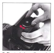
D. The standard magnifier supplied with the waist-level finder has a power of -1.5 diopters, which can be exchanged with other optional magnifiers with powers of -4.5 to +2.5 diopters. Simply rotate the magnifier frame in the counter-clockwise direction to remove. To attach the magnifier, match the white marks and rotate the magnifier frame about  $30^\circ$  in the clockwise direction.
