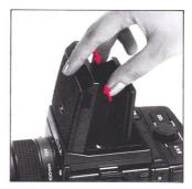
C. To close the focusing hood, first, push down the magnifier (if it is in viewing position). Next, press in both side frames, as illustrated, and, at the same time, press the front frame back towards the rear.
