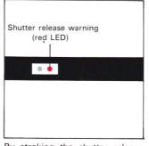
By stroking the shutter release button halfways, shutter release warning red LED and flash ready green LED illuminates in the finder display as the case may be. For detail, please refer to "14. Shutter Release Button" of GS-1 camera instruction booklet and the instruction booklet of the Speed-Light G1.
