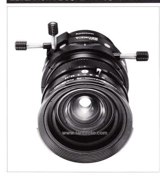
Developed with the technical cooperation of Jos. Schneider GmbH & Co., the perspective control lens has tilts of 10°, both up and down, lateral shifts to the left and right of 12mm each, rise of 12mm and fall of 10mm which can also be used in combination, thus making the optic suitable for a wide range of applications. The controls can be used for-
