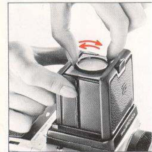
C. The standard magnifier supplied with the waist-level finder has a power of -1.50 diopters, which can be exchanged for others with Powers of +1.50, +0.50, -0.50, -2.50, -3.50 and -4.50 diopters. These optional accessories should be purchased to suit the user's eyesight, if necessary. Simply rotate the magnifier frame in the counter-clockwise direction to unscrew.
