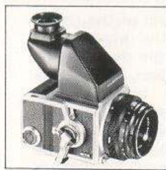
\* The Rotary Viewfinder on the ETR makes reflex view-focusing very easy, as the eyepiece end can be rotated 90° in two directions for use in both horizontal and vertical formats. Camera operations are greatly speeded up because a bright erect image, moving in the same direction as the lens, is observed for composing and focusing.
