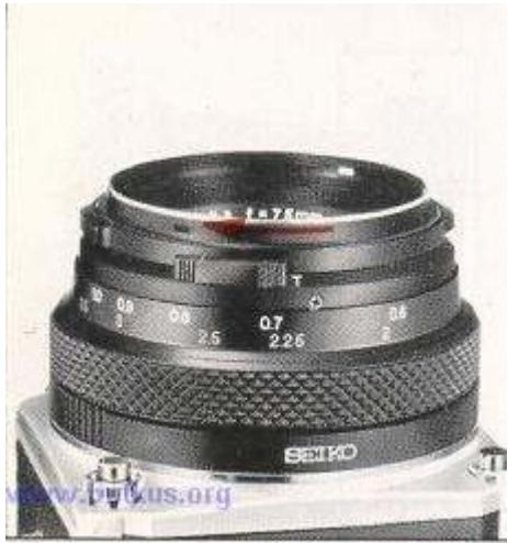
A. Time exposures are made with the time exposure lever on the lens, regardless of the setting on the shutter speed scale.
