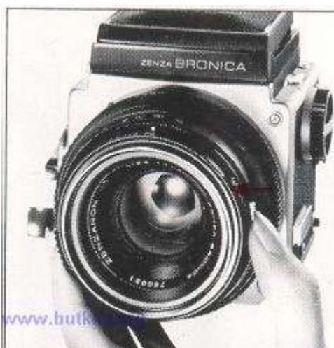
A. The aperture ring is rotated, in either direction, to set the required f/number opposite the white index dot. The aperture ring click-stops at the numbered settings. Intermediate settings are also possible.
