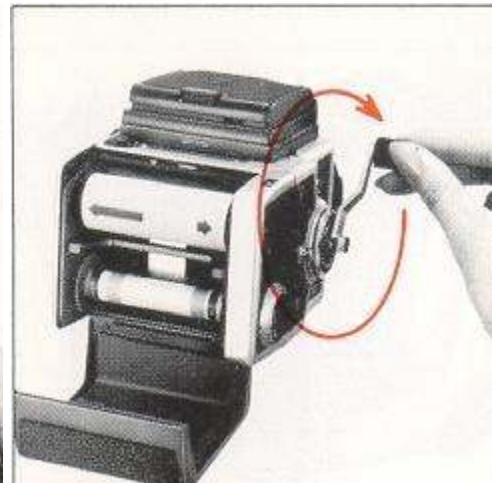
E. When the fresh film spool is properly loaded in the top spool holder, draw out the leading end of the film and turn it across the film pressure plate (on the front side of the insert). After running it down to the lower end, turn it over to the empty take-up spool. Insert the leading end of the film into the slit of the take-up spool and wind slightly so that it is securely engaged.
