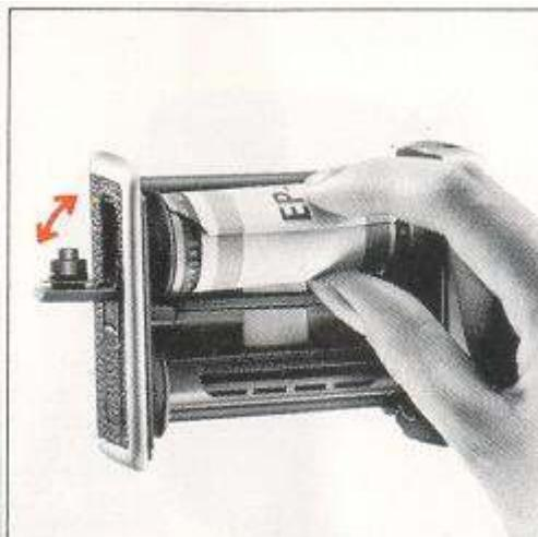
D. There are two spool holders on the film holder. The top one is for the fresh film spool while the bottom one is for the empty take-up spool. The left-side shafts of both spool holders can be opened outwards, as illustrated. Therefore, insert the right end of the spool on to the right-side shaft, which is fixed, and then close the left side holder (shaft) which will engage the spool.
