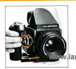
D. Stroke the film winding lever of the accessory slightly so the winding connector is in position to mesh with the attachment rod of the film winding crank on the camera body. When aligned properly, push the accessory in fully so that the two engage.
