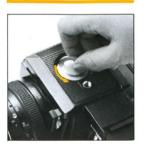
The accessory can be detached from the camera body, by simply loosening the attachment screw on the base of the accessory.
