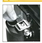
A. The hot shoe on the accessory can be used for cordless attachment of electronic flash units with suitable terminals.
