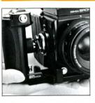
C. The camera body should be placed on the base of the accessory, after aligning the guide pins on the front end of the accessory's base to the accessory mounting guide on the base of the camera body.
