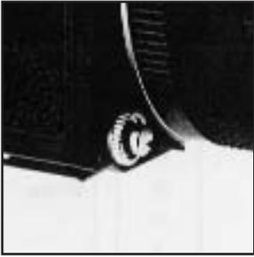
A. Depress the shutter release button with the ball of the finger. Press all the way in with a smooth and gentle action. There is no need for strength or jerky action, which will induce camera shake and affect picture sharpness.
