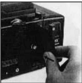
B. To remove the film back from the main body, insert the dark slide into the dark slide slit, as illustrated, with the mark on the dark slide at the top end. Push it all the way in.
