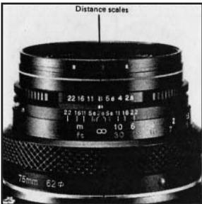
A. Distance scales on the Bronica lenses for the ETRS can be used for setting the focus on the required distance or finding the distance actually focused. Simply rotate the focusing ring and set the required distance opposite the green-colored index, which will adjust the lens for the required distance.
