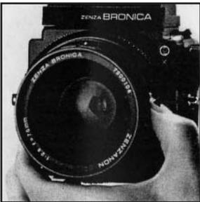
B. All Bronica interchangeable lenses for the ETRS have fully automatic lens diaphragms, which means that the focusing screen is always viewed at the full aperture, with the brightest possible image. However, depressing the depth of field preview lever will stop the lens diaphragm down to the pre-selected lens opening (aperture), permitting the photographer to check the depth of field effect on the focusing screen.
