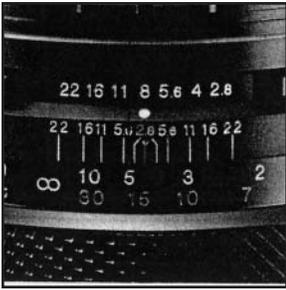
In infrared photography, some adjustments must be made in the focus in order to retain sharpness on the film, because the invisible infrared rays are longer in wavelength than the visible rays used for focusing. For infrared photography: -
