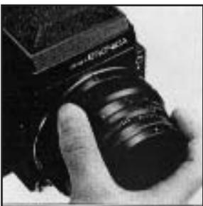
A. To attach the lens to the main body, align the red dots on the lens and the main body and then insert the lens fully into its mount. Rotate in the counter-clockwise direction until it stops, with an audible click, which will indicate that it is securely locked.
