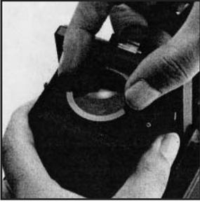
D. The standard magnifier supplied with the waist-level finder has a power of -1.5 diopters, which can be exchanged for others with powers of -4.5, -3.5, -2.5, -0.5, and +1.5 diopters. These optional accessories should be purchased to suit the user's eyesight, if necessary. Simply rotate the magnifier frame in the counter-clockwise direction to unscrew. Attach in the reverse manner.
